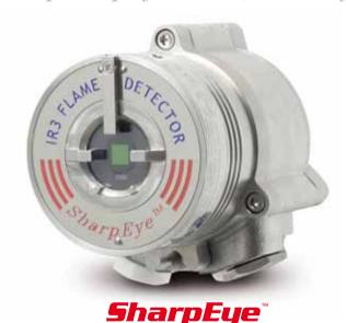
The new 40/40I Triple IR (IR3) Flame Detector detects fuel and gas fires at long distances with the highest immunity to false alarms. The 40/40I IR3 can detect a 1ft<sup>2</sup>  $(0.1m^2)$  gasoline pan fire at 215 ft (65m)in less than 5 seconds.
