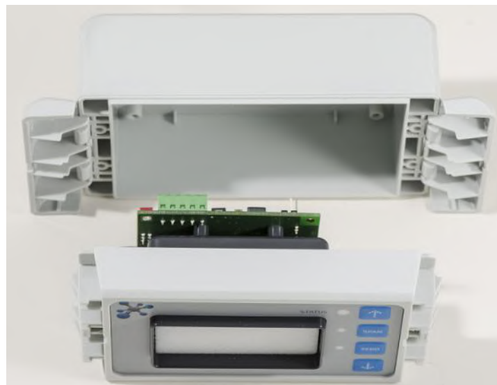
Figure 6: front casing removed
