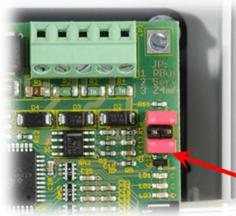
Figure 8: Link JP3 for selection of current mode (4-20mA setting is shown)
