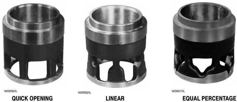
Figure 3-28. Characterized Cages for Globe-Style Valve Bodies
