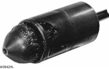
Figure 5-6. Typical Appearance of Flashing Damage
