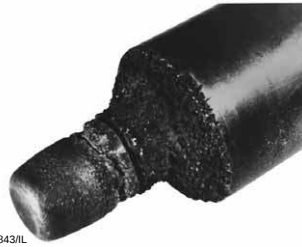
Figure 5-7. Typical Appearance of Cavitation Damage
