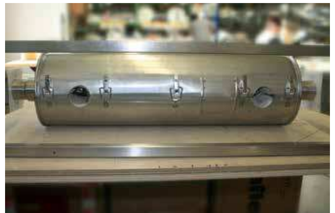
Heating jacket with sheet metal outer jacket
