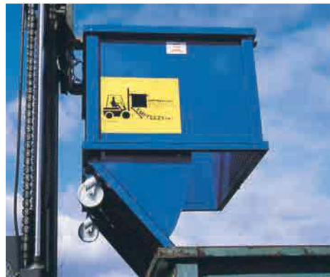
CHUTE MOUTH – FLANKED BASE TO AVOID SIDE SPILLS
