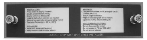
Use new, premium quality Alkaline D-Cell batteries only (Energizer E95 or Duracell/Procell MN1300). Insert batteries as shown:
