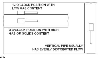
VELOCITY INCREASING DEVICES: Generally the sensor must be mounted away from flow disturbances such as valves, pumps, orifice plates, venturis or pipe inlets and discharges which tend to increase flow velocity. Velocity increasing devices often cause cavitation, or rapid release of gas bubbles, and readings both up and downstream may show much higher velocity. As a guideline, mount the sensor at least 20 diameters upstream or 30 diameters downstream from velocity increasing devices.
