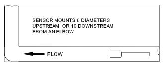
TURBULENCE INCREASING DEVICES: Elbows, flanged connections and tees tend to introduce desirable conditions of an evenly distributed flow profile with some air or gases entrained in the flow. Sensor mounting 6 pipe diameters upstream and 10 diameters downstream from these disturbances is generally optimum.
