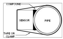
Over time temporary coupling compounds (e.g. Petroleum Gel) may gradually sag away from the sensor resulting in reduced signal strength and finally complete loss of signal. Warm temperatures, moisture and vibration will accelerate this process. Dow Corning Silicone Compound #4 as supplied with the PF D550 (and available from Micronics Limited) is recommended for semi-permanent installations.
