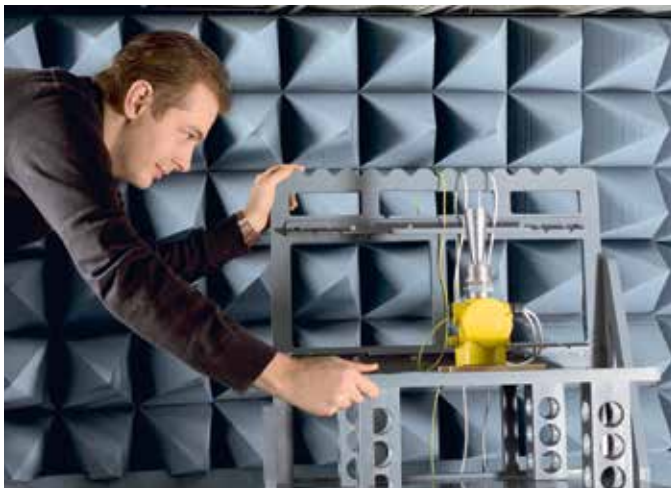
The guarantee of trouble-free quality: GTEM measuring cell (Gigahertz Transverse Electromagnetic Cell)
