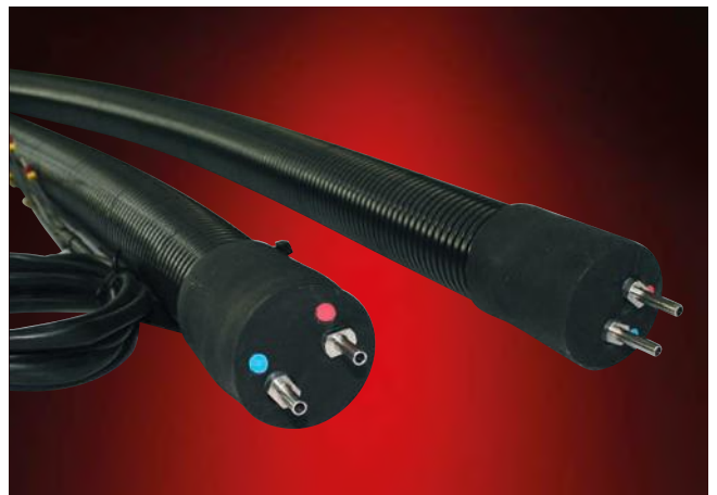
ELH/2aw-200 °C-NW6, analytic hose with 2 inner liners NW 6/8 made of Fluoropolymer with transition-free special RSL pipe stub on both sides. Holding temperature 200 °C
