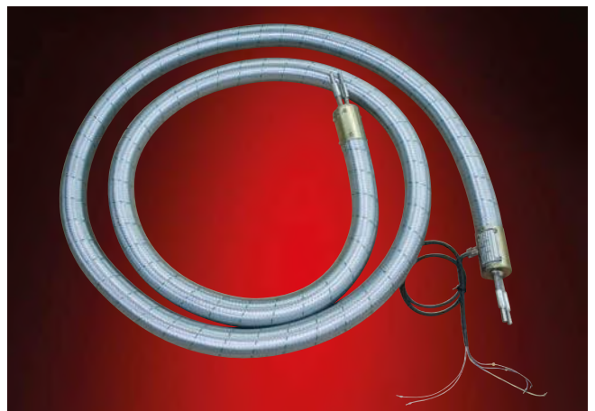
Type: ELH/2adT-150 °C-NW8/10 Heated analytic hose with 2 inner liners NW 8/10 with tread-resistant corrugated metal hose. Holding temperature: 150 °C
