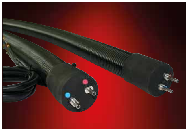
ELH/2aw-200 °C-NW6, analytic hose with 2 inner liners NW 6/8 made of PFA with transition-free special RSL pipe stub on both sides. Holding temperature 200 °C
