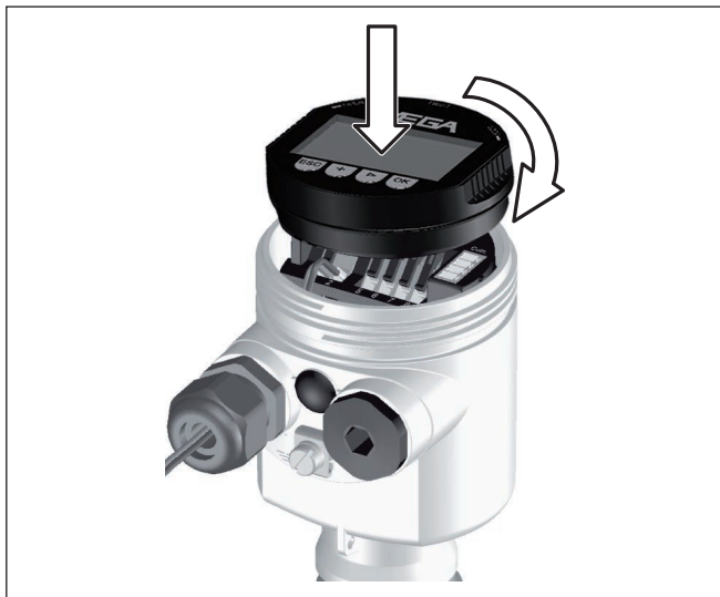
Fig. 20: Insert display and adjustment module
