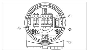
Electronics and terminal compartment, single chamber housing
