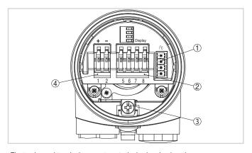
Electronics and terminal compartment, single chamber housing
