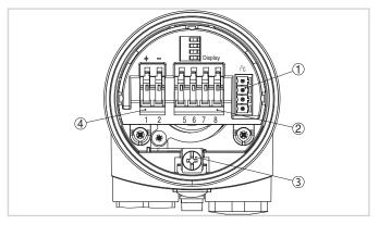
Electronics and terminal compartment, single chamber housing
