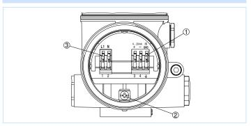
Connection compartment double chamber housing
