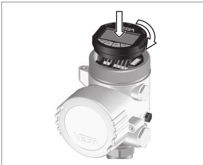
Fig. 12: Installation of the indicating and adjustment module
