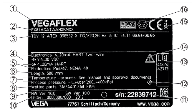
Fig. 1: Layout of the type label (example)
