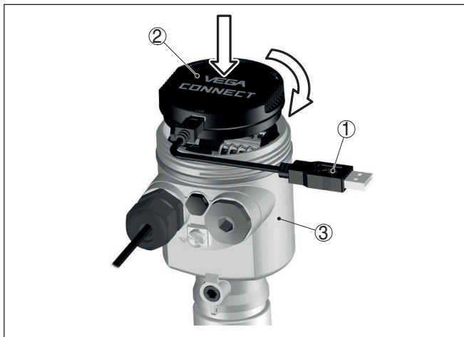
Fig. 24: Connection of the PC directly to the sensor via the interface adapter
