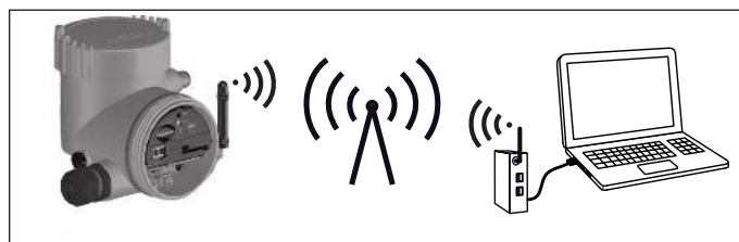
Fig. 51: Transmission of measured values and remote parameter adjustment of the sensor via mobile phone network.
