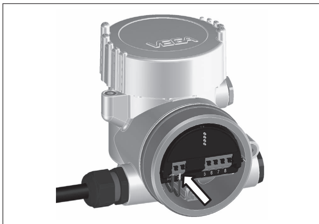
Fig. 24: Connection steps 5 and 6 - Double chamber housing
