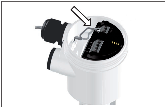
Fig. 23: Connection steps 5 and 6 - Single chamber housing
