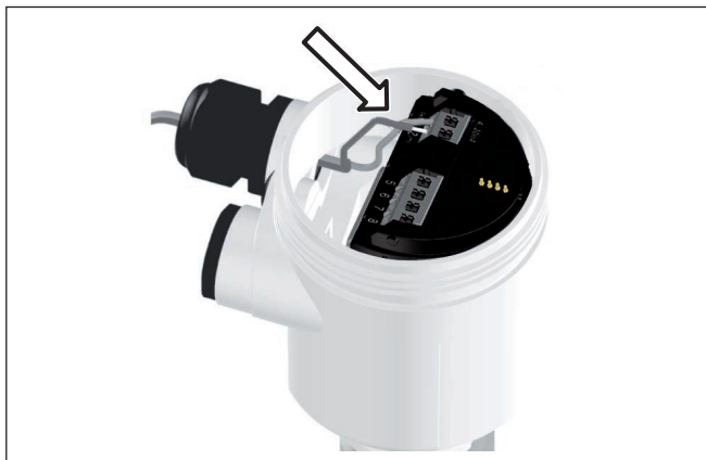
Fig. 6: Connection steps 5 and 6 - Single chamber housing
