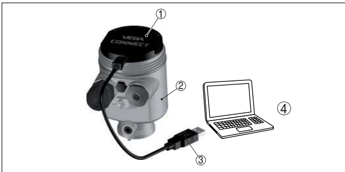
Fig. 30: Connection of the PC via VEGACONNECT and USB
