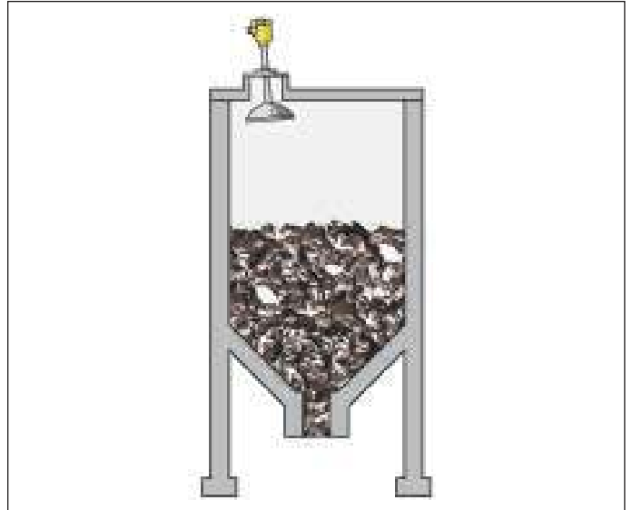
Fig. 18: Level measurement in a clinker silo with VEGAPULS 68
