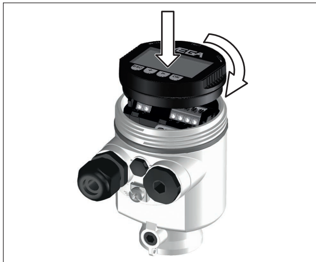
Fig. 7: Insertion of the display and adjustment module with single chamber housing
