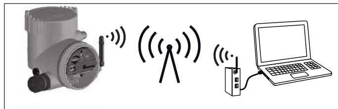
Fig. 33: Transmission of measured values and remote parameter adjustment of the sensor via mobile phone network.
