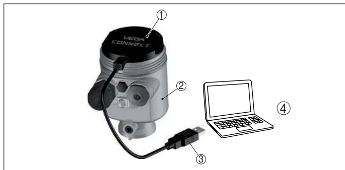
Fig. 34: Connection of the PC via VEGACONNECT and USB
