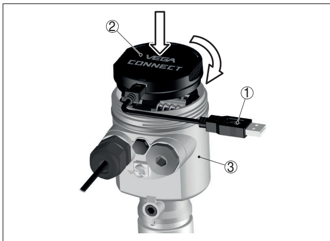
Fig. 21: Connection of the PC directly to the sensor via the interface adapter
