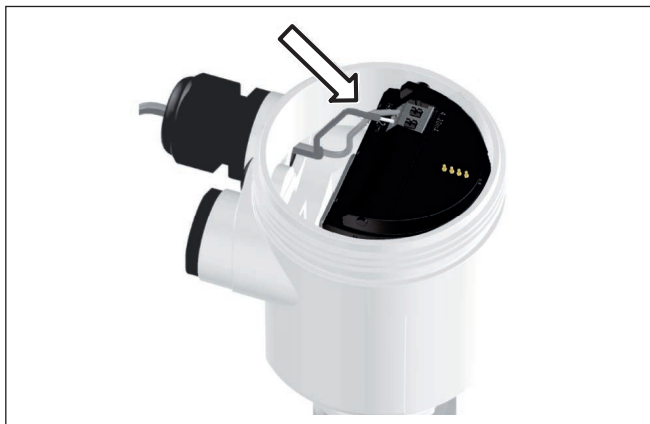
Fig. 3: Connection steps 5 and 6 - Single chamber housing
