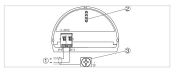
Electronics and terminal compartment, single chamber housing
