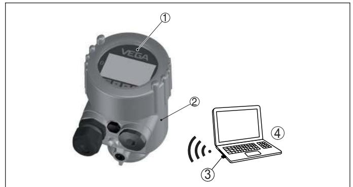
Fig. 47: Connection of the PC via Bluetooth adapter
