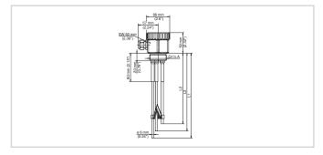
Conductive probe EL 3 L1-3Probe length
