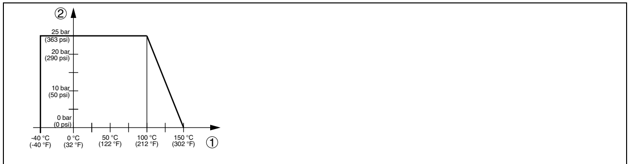
Fig. 19: Product temperature - Process pressure
