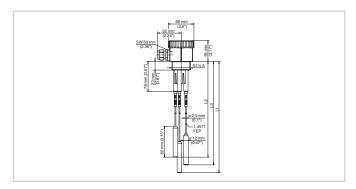
Conductive probe EL 6 L1-3Probe length
