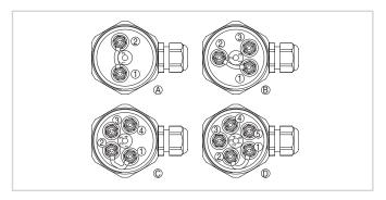
Connection compartment of the probe - 220  $\mbox{k}\Omega$  resistance between terminals 1 and 2
