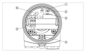
Oscillator - Contactless electronic switch
