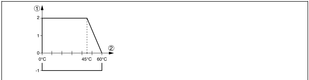
Fig. 14: VEGACAP 69 - process pressure - Process temperature (flange of PP)
