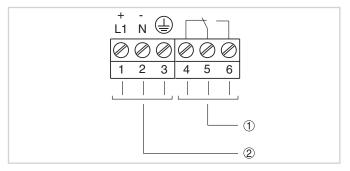
Electronics with relay output
