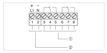
Electronics with relay output
