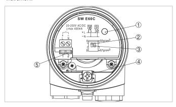
Electronics and terminal compartment, single chamber housing
