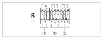
Wiring plan, single chamber housing
