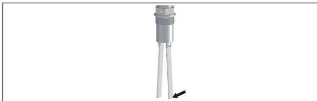
Fig. 29: Max. lateral load alongside fork side (narrow fork side)
