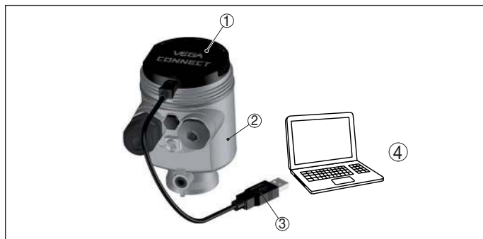
Fig. 27: Connection of the PC via VEGACONNECT and USB
