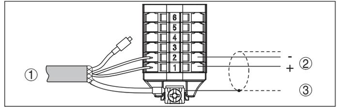
Fig. 22: Wiring plan VEGABAR for 4 ... 20 mA, 4 ... 20 mA/HART
