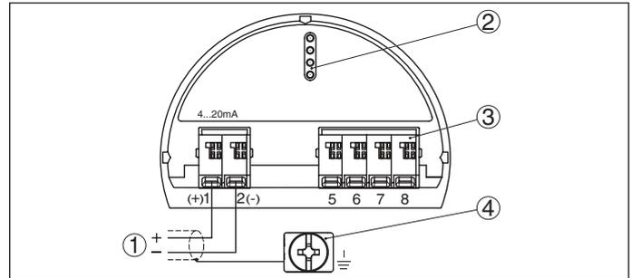
Fig. 20: Electronics and terminal compartment, single chamber housing
