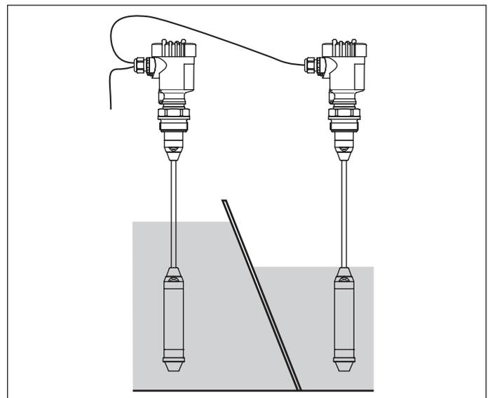
Fig. 9: Electronic level difference measurement through Master/Slave combination
