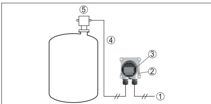
Fig. 38: Connection of VEGADIS 82 to the sensor
