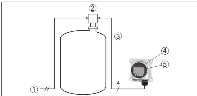
Fig. 37: Connection of VEGADIS 81 to the sensor
