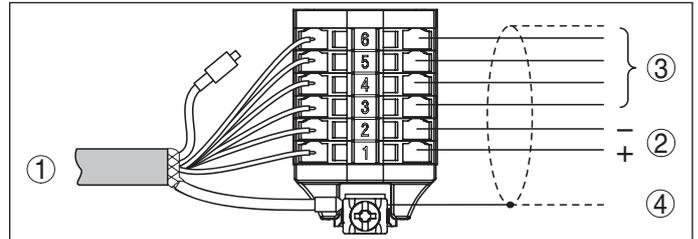
Fig. 26: Wiring plan VEGABAR for 4 ... 20 mA/HART Pt 100
