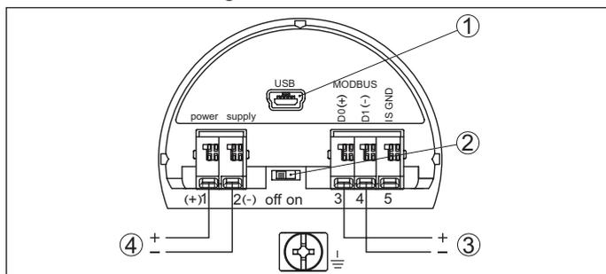
Fig. 31: Terminal compartment
