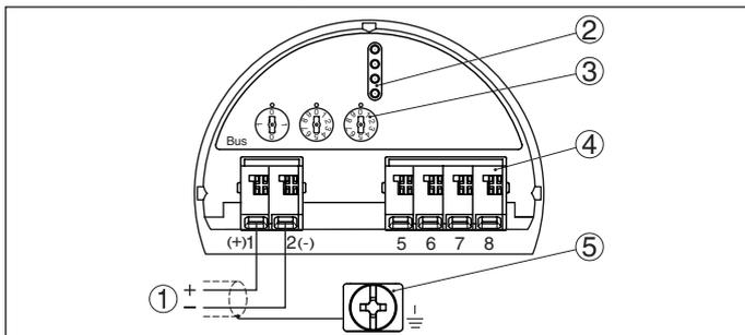
Fig. 27: Electronics and terminal compartment, single chamber housing
