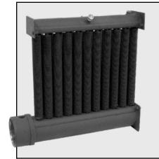
The *ExCaliber*™ vacuum sealed liquid-to-air heat exchanger core is constructed using rugged, copper-free, roll-formed aluminum fins and protected by a pressure relief device, automatic reset high limit, and a back-up manual reset high limit.
