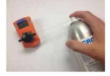
This is purely for bump testing and cannot be used for calibrations. For further information, Contact Crowcon.
