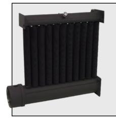
The *ExCaliber™* vacuum sealed liquid-to-air heat exchanger core is constructed using rugged, copper-free, roll-formed aluminum fins and protected by a pressure relief device, automatic reset high limit, and a back-up manual reset high limit.
