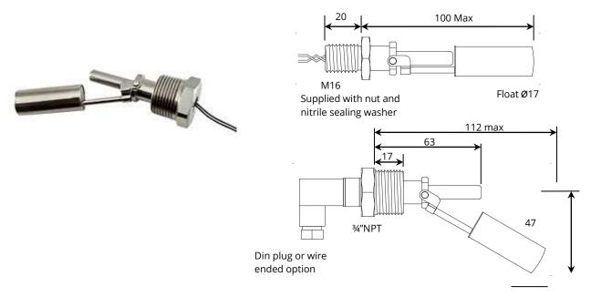
The 80 Series is a small horizontally mounted liquid level sensor designed for high temperature/high pressure operation and sensing chemically aggressive liquids. The design provides a highly cost effective solution where high reliability in a demanding environment is called for.
