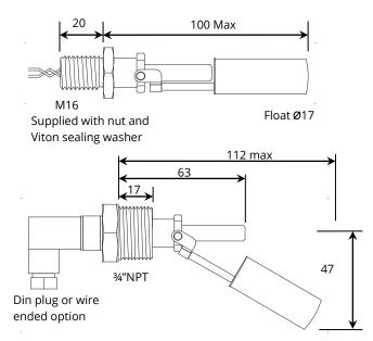
The 80 Series is a small horizontally mounted liquid level sensor designed for high temperature/high pressure operation and sensing chemically aggressive liquids. The design provides a highly cost effective solution where high reliability in a demanding environment is called for. The high temperature version of the 80 series has the added benefit of being able to operate in temperatures exceeding the standard limit of 120°C and can operate in temperatures of up to 200°C.
