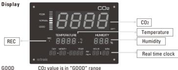
CO2 value is in "GOOD" range NORMAL CO2 value is in "NORMAL" range CO2 value is in "POOR" range P00R Unit of relative humidity °C/°F Unit of temperature (Celsius/Fahrenheit) REC Blinking in automatic logging mode
