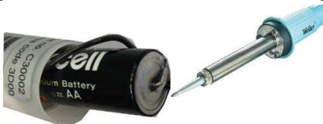
Figure 13: Unsoldering the battery
