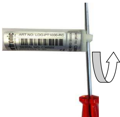
Figure 11: Unscrew cover with screwdriver
