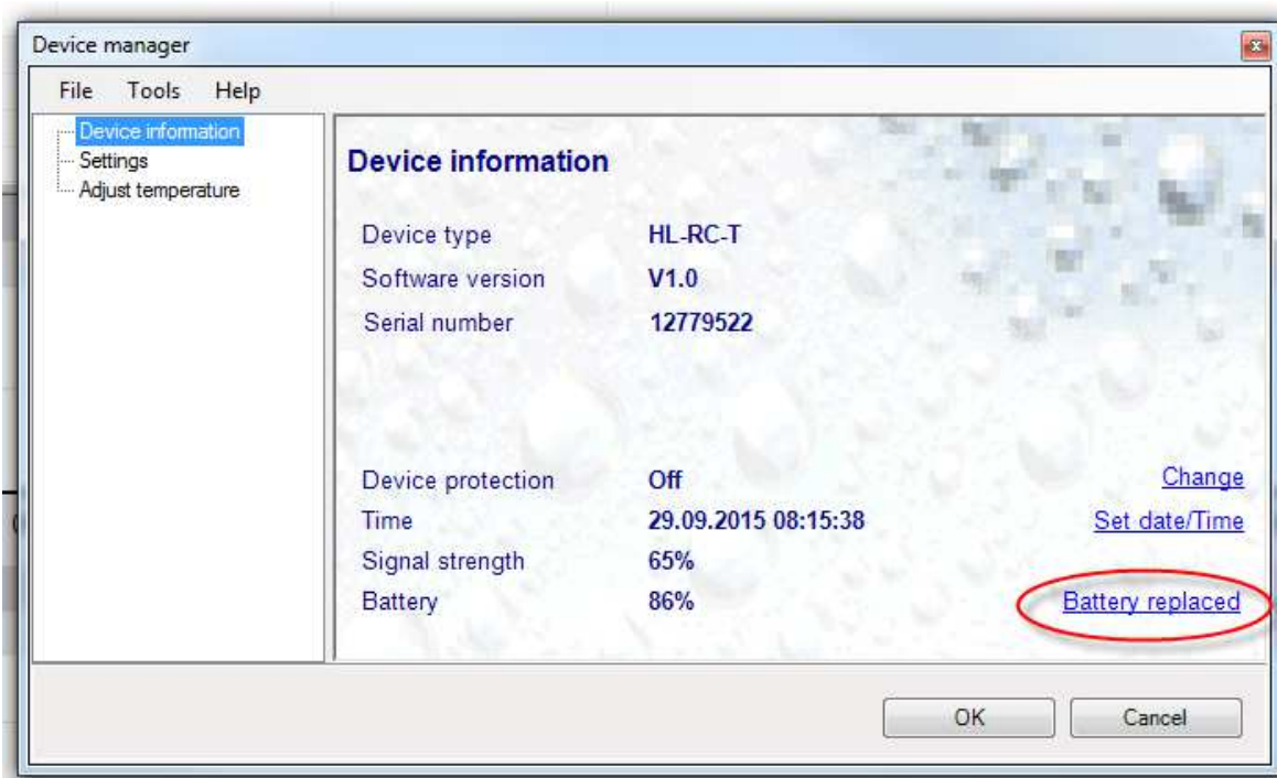
Figure 16: Setting the time after a battery change
