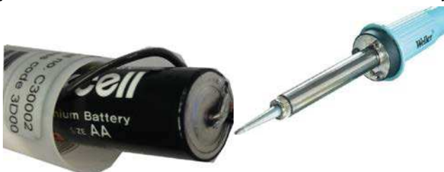
Figure 13: Unsoldering the battery
