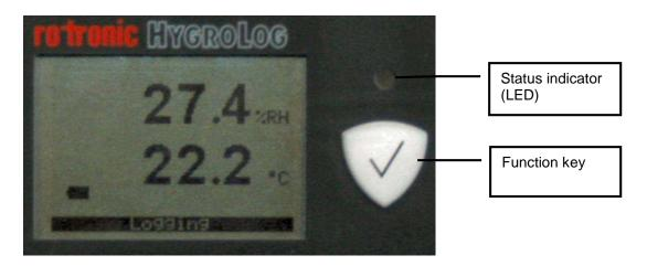
The LC display has a backlight which can enabled or disabled as part of the data logger configuration. When the backlight is enabled, it turns on for a few seconds after pressing on the function key.
