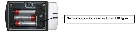
Use cable AC3006 to connect the data logger to a USB port of the HW4 PC. Start HW4 and discover the data logger by selecting with the mouse the following command in the menu bar: Devices and Groups > Search for Master Devices > USB Masters.
